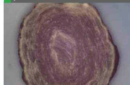
Fig. 6: Cross-section of a single fertilizer granule at different magnifications showing colourant performance and distribution
